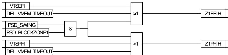
Allow Zone 2 to be inhibited by the same; Power Swing, VTS, or Vmem timed out.
