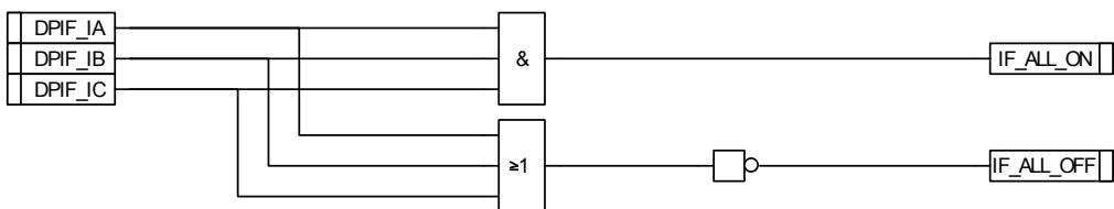
Next, we generate the latch control signals for use by the distance module output latches - first the latch enable
